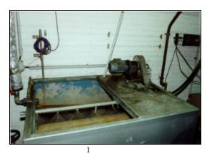
"The problem used to be that deposits started to build up after only a short operating time that it was impossible to remove" Mr. Sandor remembers. The expensive result was that the sieve had to be replaced frequently. Nowadays, the slurry is removed at intervals of four to five weeks with a high-pressure cleaning jet, and the sieve does not need to be replaced at all.
